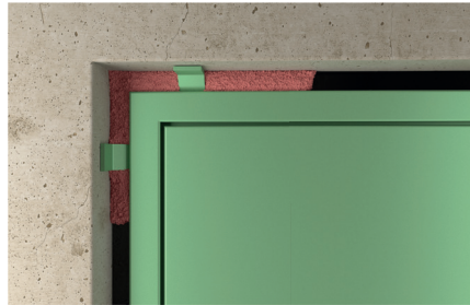
Back filling material
