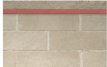
Construction joint application
