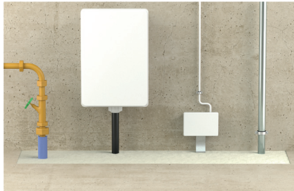
Mixed penetration through the floor
