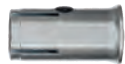
Hammerset anchor EA II, with reduced anchorage depth h_{ef} 25 mm and a black fixing point which prevents the anchor from falling out of the drill hole.
