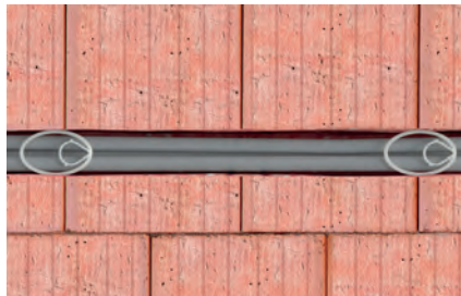
Cable fixing in wall slots > 30 mm
