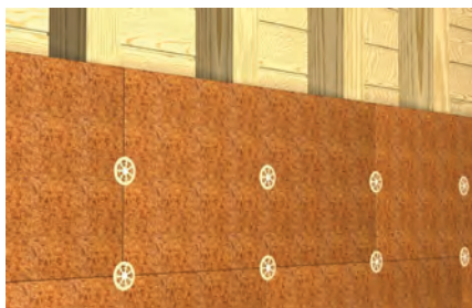
Fixing of wooden soft fibre boards on solid wood
