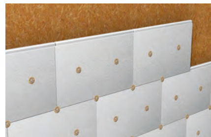
Attachment of polystyrene boards on OSB-panel
